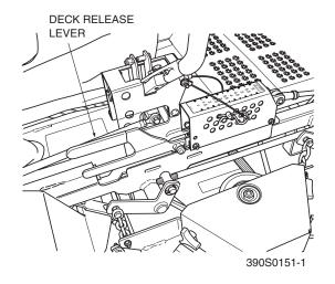
Figure 4-6. Deck Release Lever
